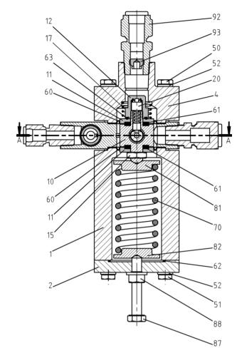
6.2 Spare parts drawing for imperial HON640a pilot with diaphragm measuring unit
